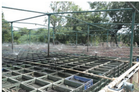
Wastewater being purified through earthworm farming
