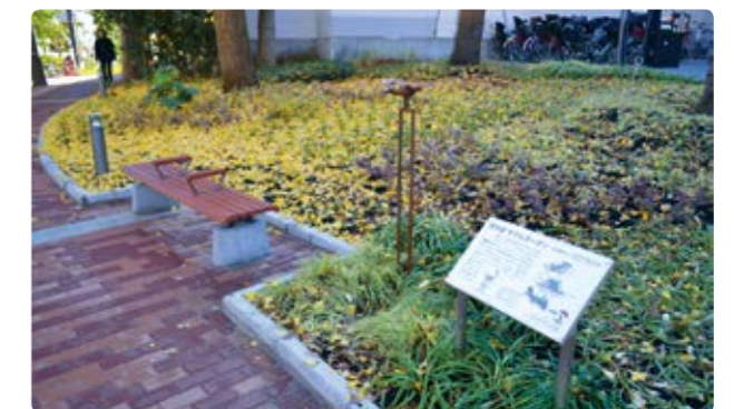
Rain Garden™ Rainwater is contaminated with substances contained in exhaust gas and involves the risk of disrupting the ecosystem if it flows directly into seas and rivers. Rain Garden™ reduces the negative impact on the ecosystem by allowing rainwater to penetrate into the ground and purifying it.
