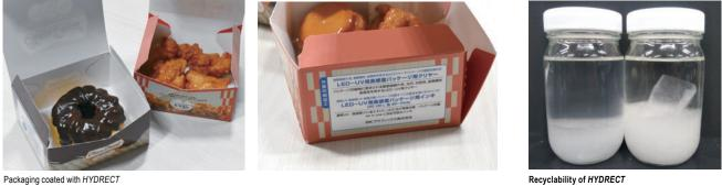
Recyclability of HYDRECT Paper coated with HYDRECT dissolves completely in chemicals (left), while that laminated with polyethylene does not (right)
