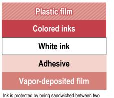
Ink is protected by being sandwiched between two layers of film.
