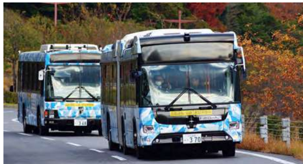
Experimental autonomous vehicles driving in formation on public roads in Higashihiroshima (front: articulated bus, rear: large bus)
