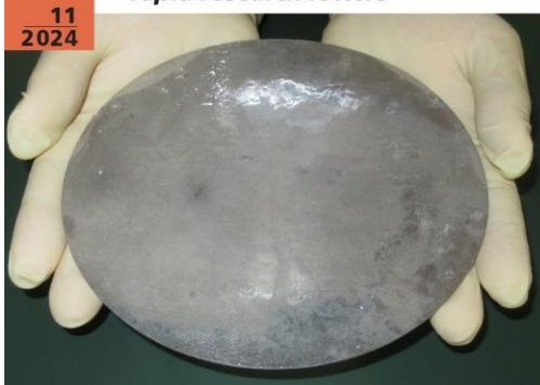
Large GaN seed crystal on the inside cover
