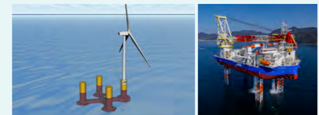
Image of semi-submersible floating foundation developed by Japan Marine United for the Southern Akita Offshore Project Jack-Up Vessel built by Japan Marine United
