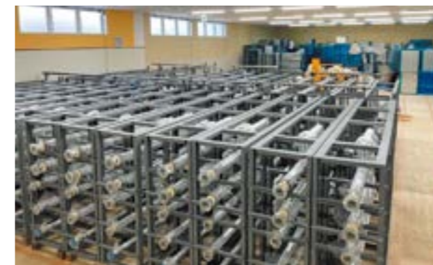
Processed piping unit
