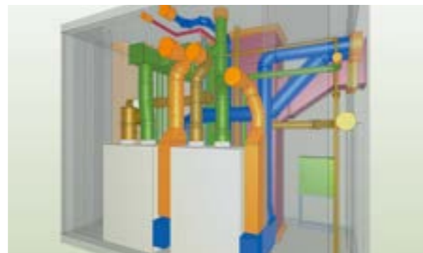
Existing equipment location plans are created using point cloud data from 3D measurement technologies
