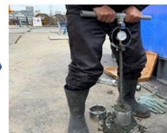
Quality Inspection (Cone Penetration Test)
