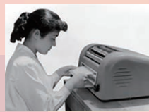
The Ricopy 101, Japan's first desktop diazo-wet copier to integrate exposure and development (1955)
