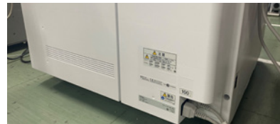
Exterior cover with recycled plastic from horizontal recycling
