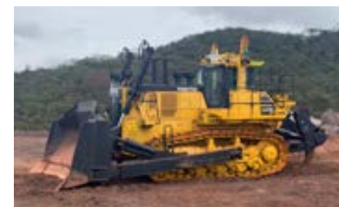
Bulldozer D375Ai-8 remotely operated at Minas-Rio iron mine in Brazil
