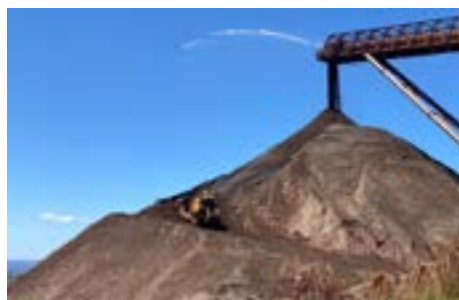
Remotely operated bulldozer for stockpile operations at a mine site.
