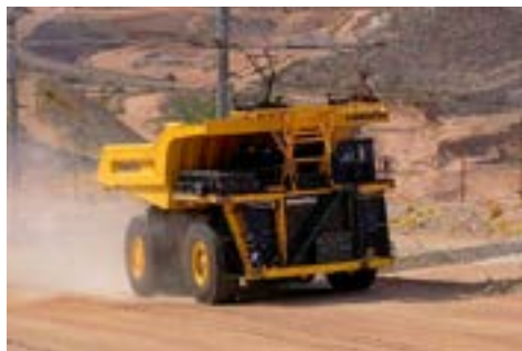
Battery-electric trolley mining truck (Concept machine)
