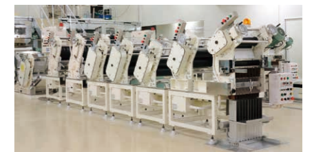
DDM continuous noodle-sheet press roller Equipped with direct drive motor (DDM) with motor and roll directly connected. Waved rolls create a handmade-like noodle texture
