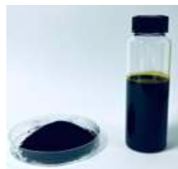
Recovered carbon black (left) and tire-derived oil (right)
