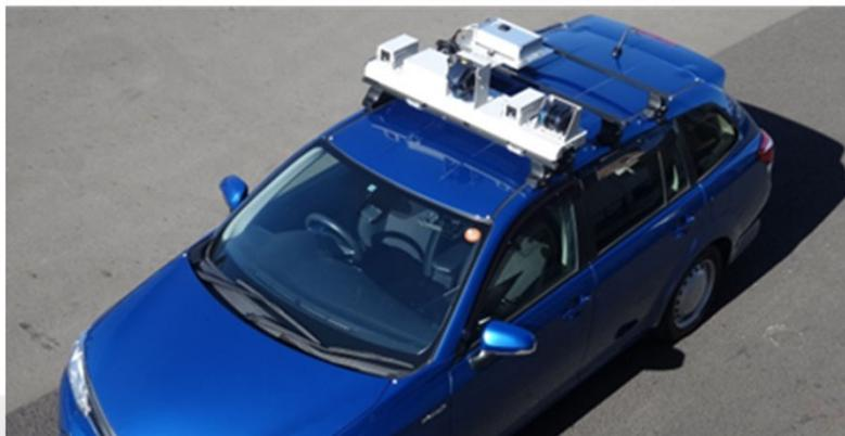
**Road Surface Properties Measuring Vehicle**
