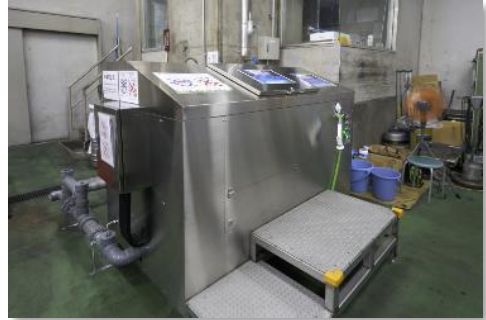
Fully automated vanishing-type food waste disposers
