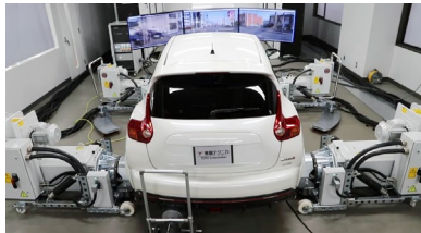
ROTOTEST® Energy™ (hub coupled chassis dynamometer)
