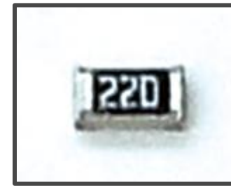
Letter/shape imaging (Small chip parts; about 1mm)
