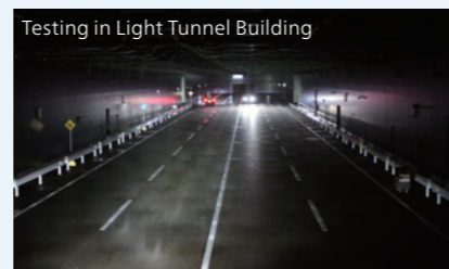
Light Tunnel Building: One of the world's longest indoor test facilities, it can accurately reproduce the natural environment, including rainfall, fog, and other conditions, allowing us to conduct verification tests on real vehicles day and night
