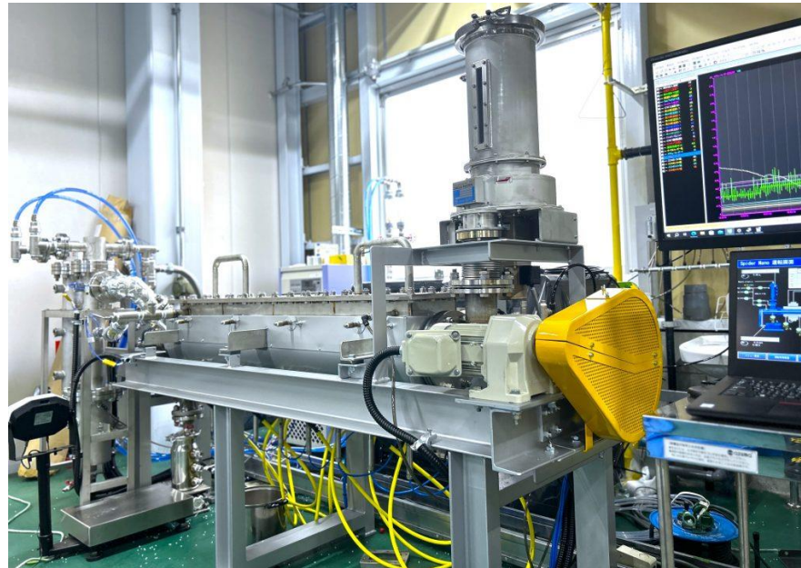
Microwave-based continuous chemical recycling demonstration unit
